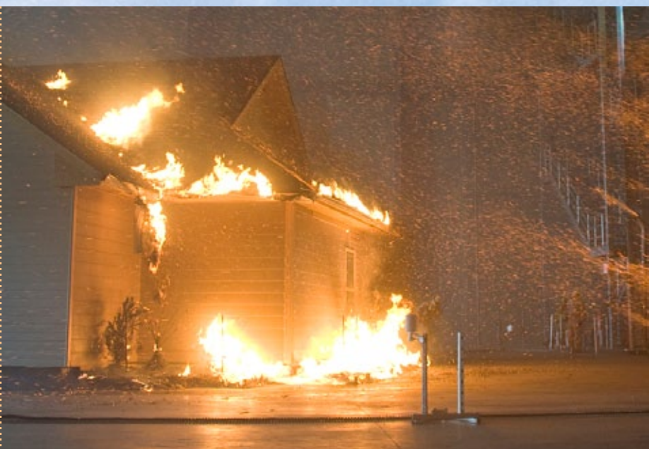
SRNL took part in a media demonstration given during Wildfire Media Day in March at the Insurance Institute for Business and Home Safety to illustrate that embers, rather than direct flame contact, cause many buildings to burn during wildfires.
